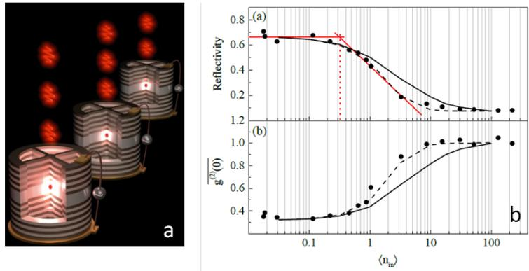
**Fig. 1:** (a) Artist view of the quantum-dot cavity devices performing as near optimal atom-photon interfaces. (b) Reflectivity (top) and second order intensity correlation function (bottom) of the directly reflected light as a function of the incident photon number (pulsed excitation).
