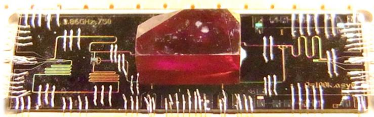
**Fig. 1:** Hybrid circuit with superconducting resonators and qubits coupled to an ensemble of NV centers in diamond.
