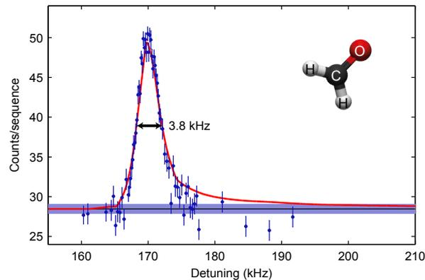
**Fig. 1:** Doppler-limited rotational transition line between  $J = 4$  and  $J = 5$  of trapped formaldehyde at 364 GHz. Measured data shown in blue and theoretical lineshape in red. Theory takes into account the energy distribution of the molecules and the electric field distribution in the trap.
