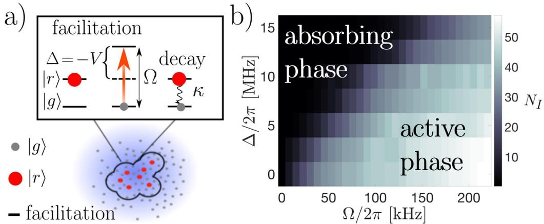
**Fig. 1:** (a) Microscopic processes leading to an absorbing state phase transition in a gas of cold Rydberg atoms with ground state  $|g\rangle$  and excited state  $|r\rangle$ : facilitation (characterized by the van der Waals interaction  $-V$  matching the detuning  $\Delta$  for off-resonant excitation) and decay at rate  $\kappa$ . (b) Phase diagram of the experimental system: stationary number of Rydberg excitations  $N_I$  versus driving frequency  $\Omega$  and detuning  $\Delta$ .
