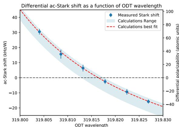
**Fig. 1:** (Preliminary) ac-Stark shift as a function of trap laser wavelength. The blue band is the calculated differential polarizability from reference [5] with its uncertainty range (rescaled to the data). The leading uncertainty in this calculation is a constant offset caused by the continuum contribution to the polarizability. The dashed line is the calculation with this offset fitted to the data.
